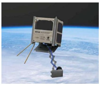
centimeter cube weighing 1 kilogram, covered on all sides by coated birch plywood from WISA plywood. Nine small solar cells will power the satellite, which will orbit at an altitude of 500 – 550 kilometers.
